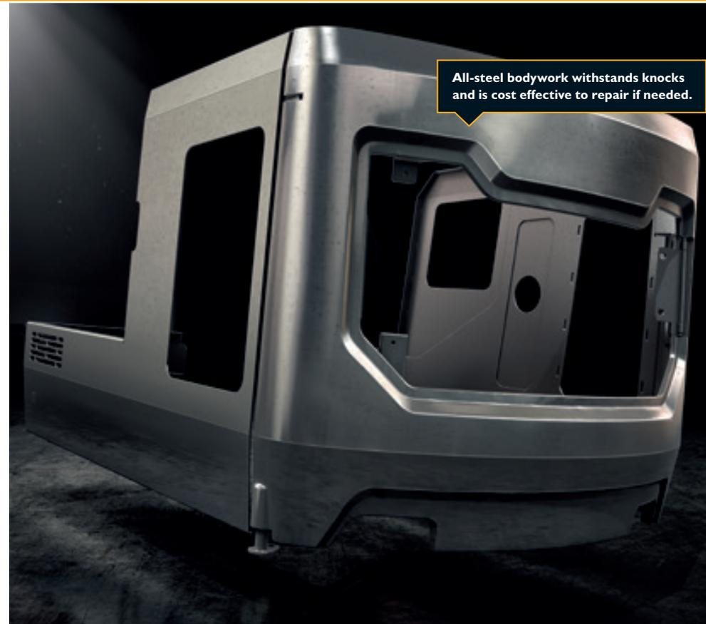
All-steel bodywork withstands knocks and is cost effective to repair if needed.
