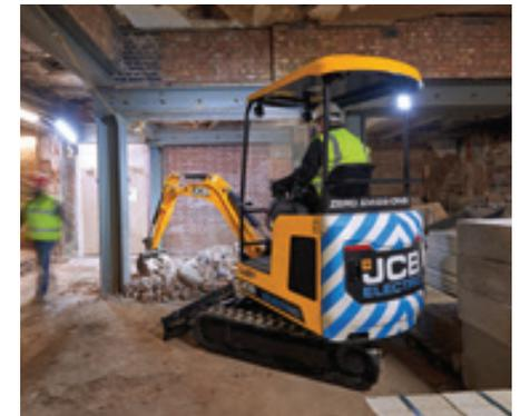
4 Auto-idle reduces the engine speed (RPM) when the machine is idle for a set amount of time, to preserve battery charge.
