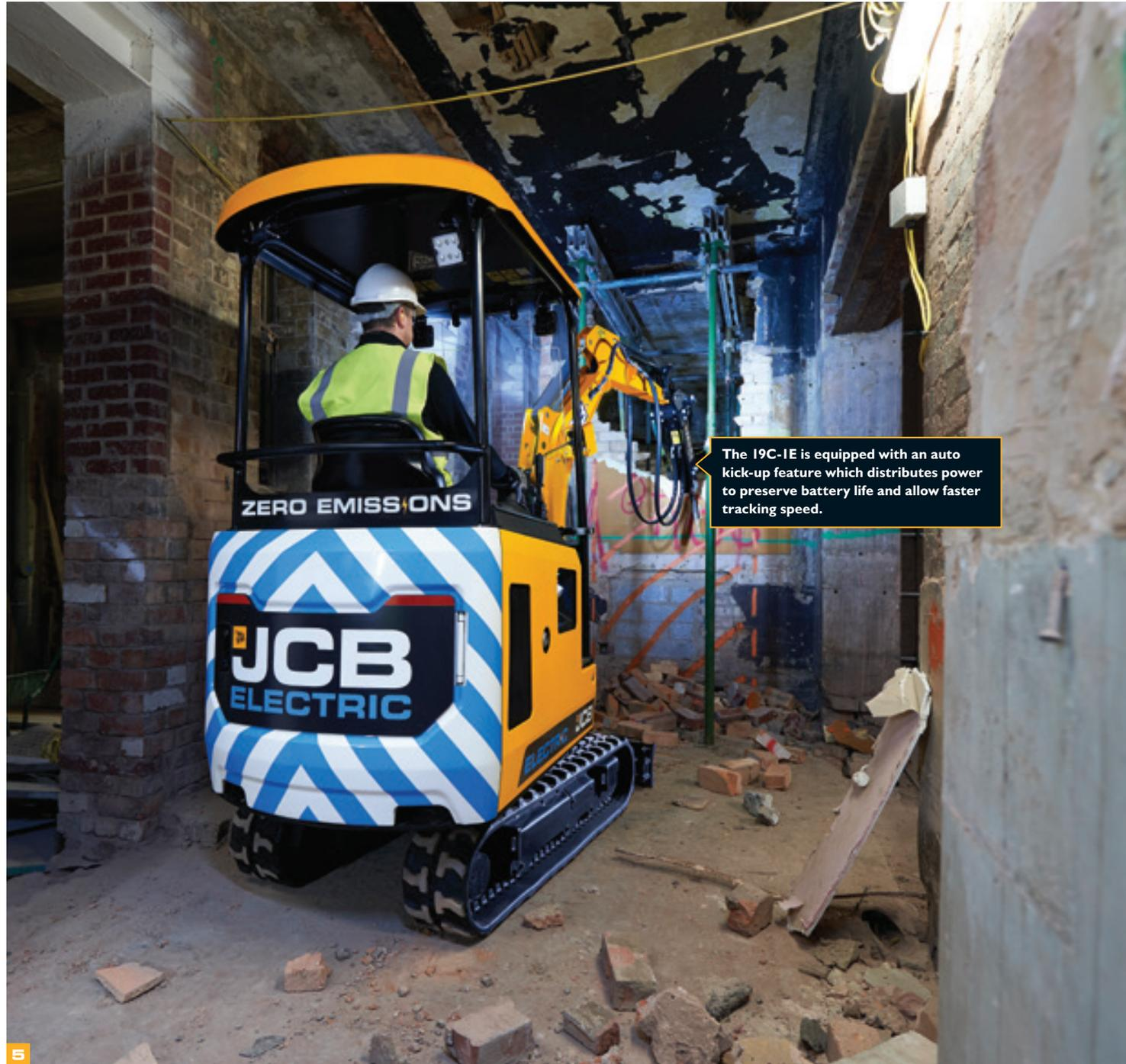
The 19C-IE is equipped with an auto kick-up feature which distributes power to preserve battery life and allow faster tracking speed.
