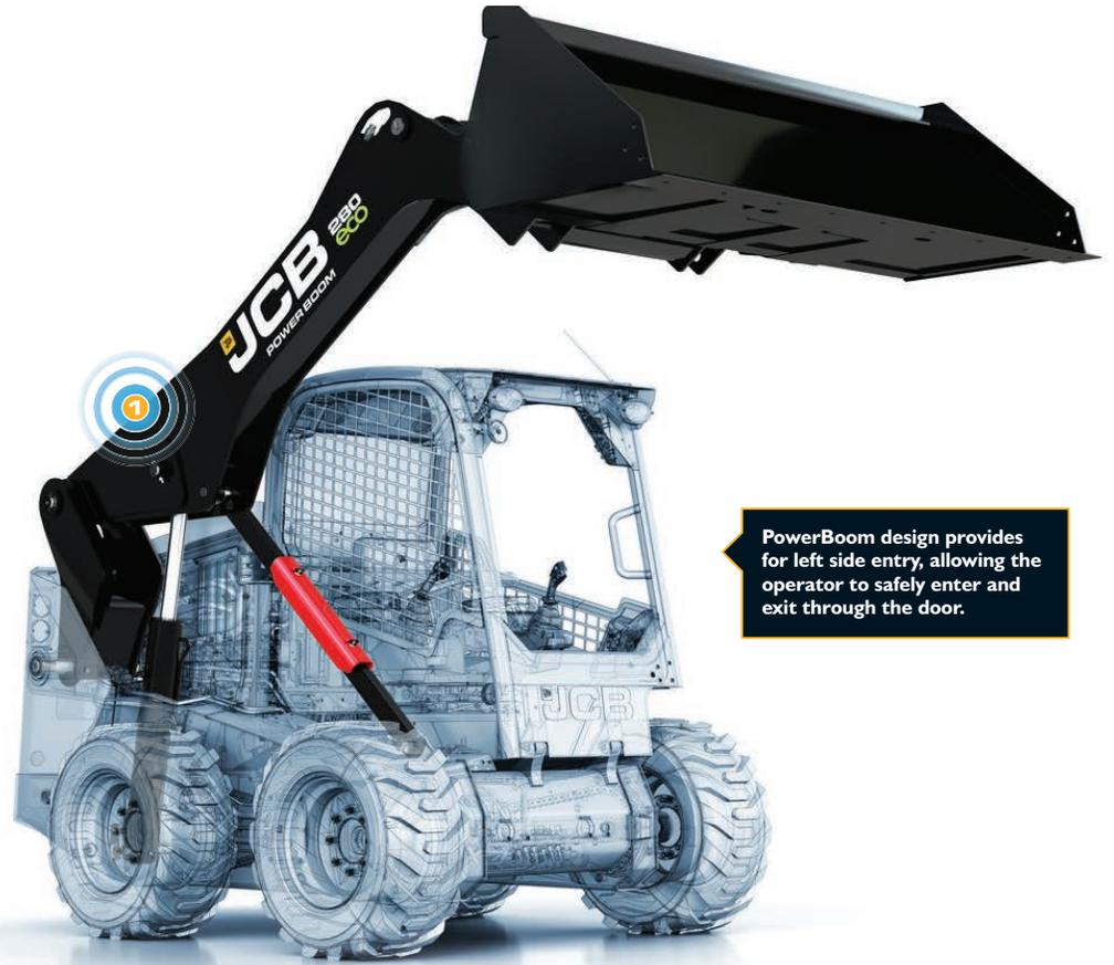
PowerBoom design provides for left side entry, allowing the operator to safely enter and exit through the door.
