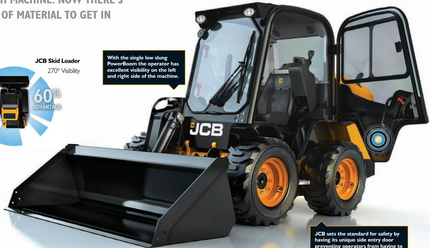
JCB sets the standard for safety by having its unique side entry door preventing operators from having to climb over dangerous attachments to enter the machine.
