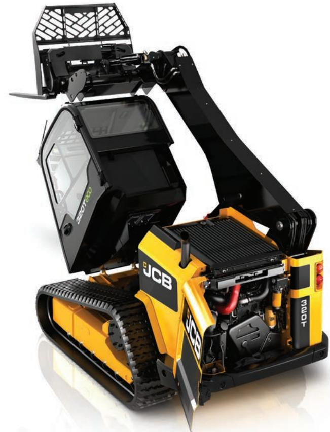
4 Tilting cab design enables easy access during more detailed machine maintenance.
